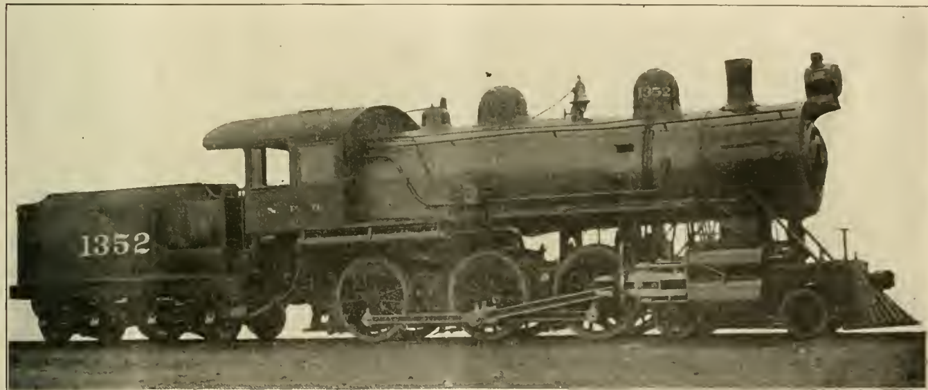
COMPOUND TEN-WHEEL, FAST FREIGHT ENGINE.—NORTHERN PACIFIC RAILWAY.
